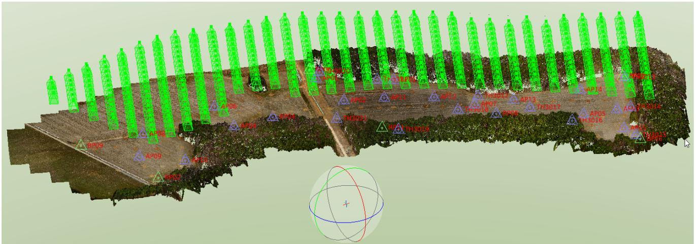
FIG.1: R-2582A ROBINSON 2 PIT - ORIGINAL FLIGHT DENSE POINT CLOUD, CONTROL POINTS, CHECK POINTS, & NADIR FLIGHT LINES
